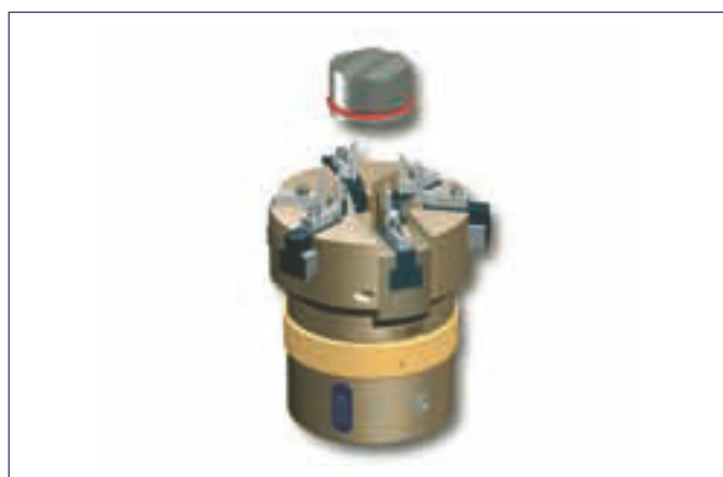
4. Retraction of the whole gripper. The o-ring is completely inserted in the groove now.
